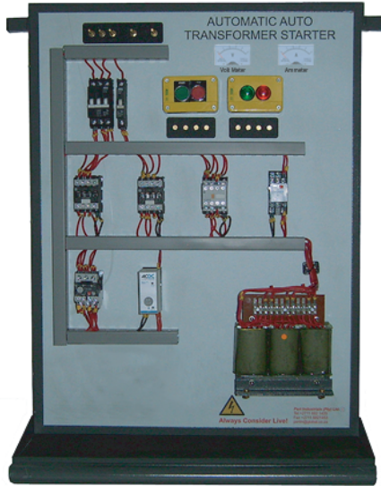
Auto Transformer Starter
